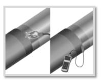
Step 6: Using medium to high intensity flame, pre- heat and activate the surface to be covered with heat shrink sleeve and min 2" on each side of the sleeve to a minimum temperature of 150°F. The flame shall be kept perpendicular to the surface of the pipe and casing during preheating. Check the temperature around entire circumference of the pipe with a touch probe.
